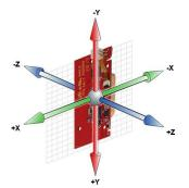
The module contains an optional 3D accelerometer (up to 16g), which can be used for a variety of custom specific (M2M) applications. Accelerometers are useful for measuring movement, speed, g-forces and vibration of the object. The accelerometer and advanced embedded firmware enables a very low-power battery solution.
